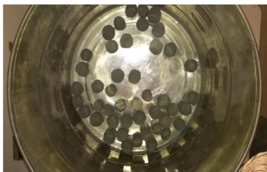
Figure 1. Geopolymer pebbles after steam curing
